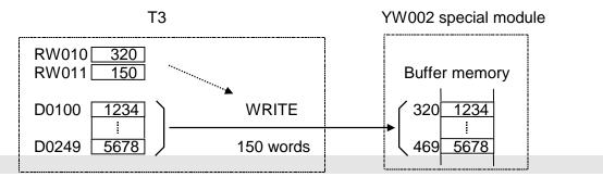
Note 1) The special module can be designated not only by the assigned register, but also by the mounting position. The mounting position is designated by a constant data for the operand C as follows.
